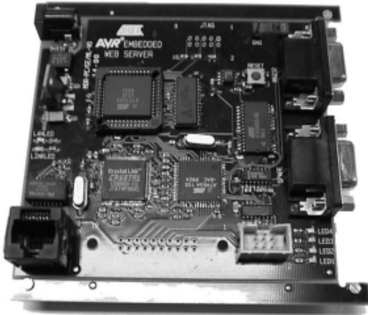
Figure 1. AVR Embedded Web Server
